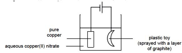
The experiment failed and no copper was deposited on the plastic toy.
